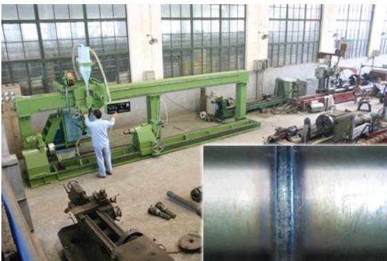
自主研发的万向轴专用埋弧焊机 Submerged arc welding and gas shielded welding machines
