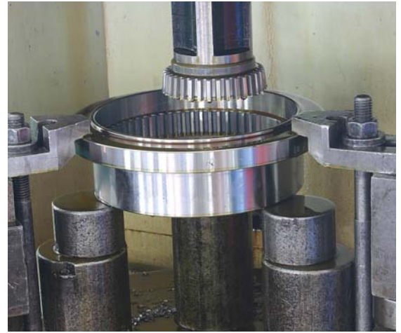
数控设备加工内外齿 Tooth profiling by CNC machine
