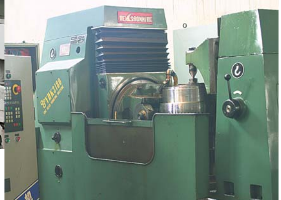
数控设备加工内外齿 Tooth profiling by CNC machine
